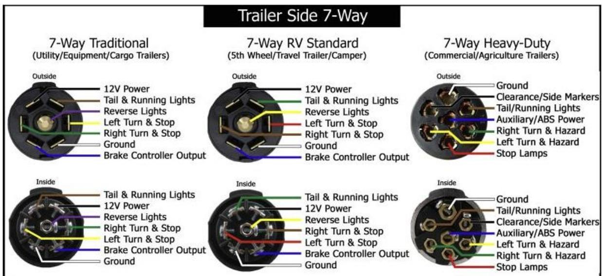
Note: To ensure your tracker is wired correctly, we recommend using a circuit tester to verify each pin's function. Wire colors can vary and are not always reliable indicators of function. Incorrect wiring can potentially damage electrical components.
